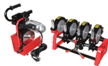
SHDS 160 Y A4 (40 - 160 mm) Manual Butt Fusion Welding Machine
